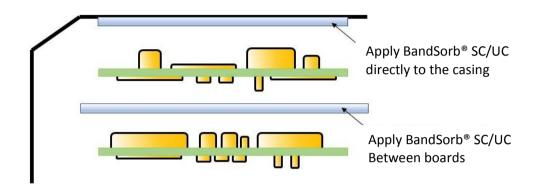
**Example 2** – To suppress noise radiation (reflected noise) from the opening of shield or casing.
