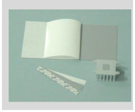
E-Phase 7300 is a thermally conductive phase change material having a softening temperature of 55°C. The liquid phase of the material can fill interface irregularities with much higher efficiency than traditional gap filler. On the other hand, it is a solid at room temperature and can be handled easily during installation.
